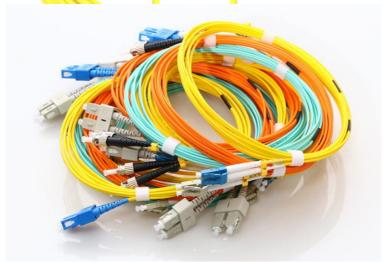
Single mode Multimode Mode UPC Polish APC PC ≤0.20dB ≤0.30dB ≤0.20dB Insertion Loss Return Loss ≥50dB ≥60dB ≥30dB Test Wavelength 1310/1550nm 850/1310nm
